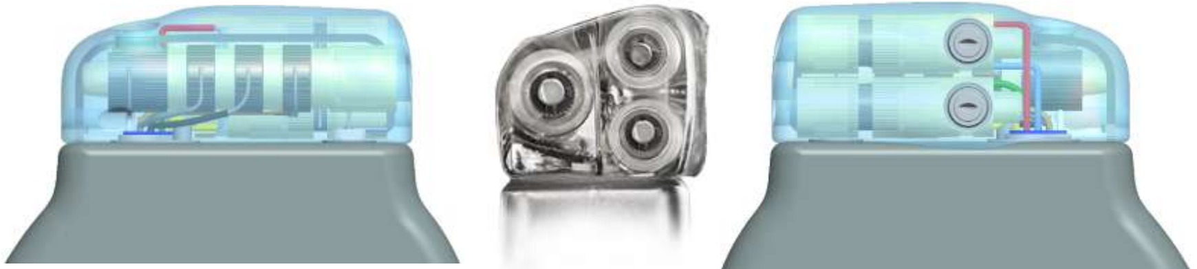
New DF4 Header for CRT-D Devices (3 setscrews)
