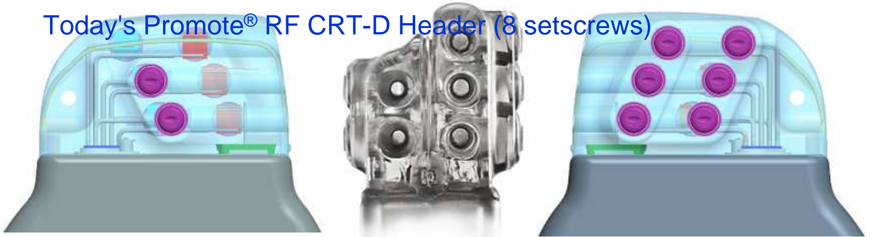
New DF4 Header for CRT-D Devices (3 setscrews)
